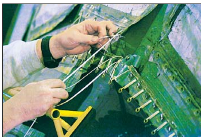
At left, Scott Babbo applies a decal stripe to the bottom of the new Goodyear blimp. Above, Jared Haren laces the nose section onto the envelope inflated with helium.
