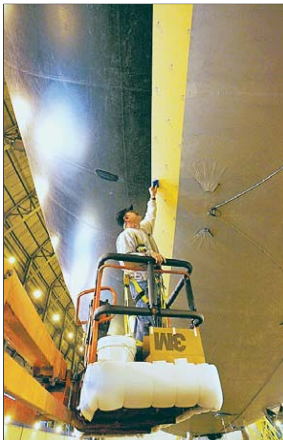
At left, Scott Babbo applies a decal stripe to the bottom of the new Goodyear blimp. Above, Jared Haren laces the nose section onto the envelope inflated with helium.
