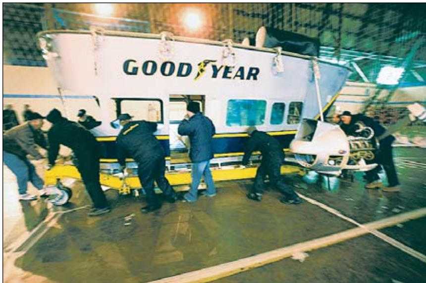
Gondoliers of Goodyear Above, crew members maneuver the Goodyear blimp gondola into position Thursday beneath the envelope at the Wingfoot Lake hangar. At right, Tim Cartell adjusts sand-filled ballast bags. The new airship has not been named.
