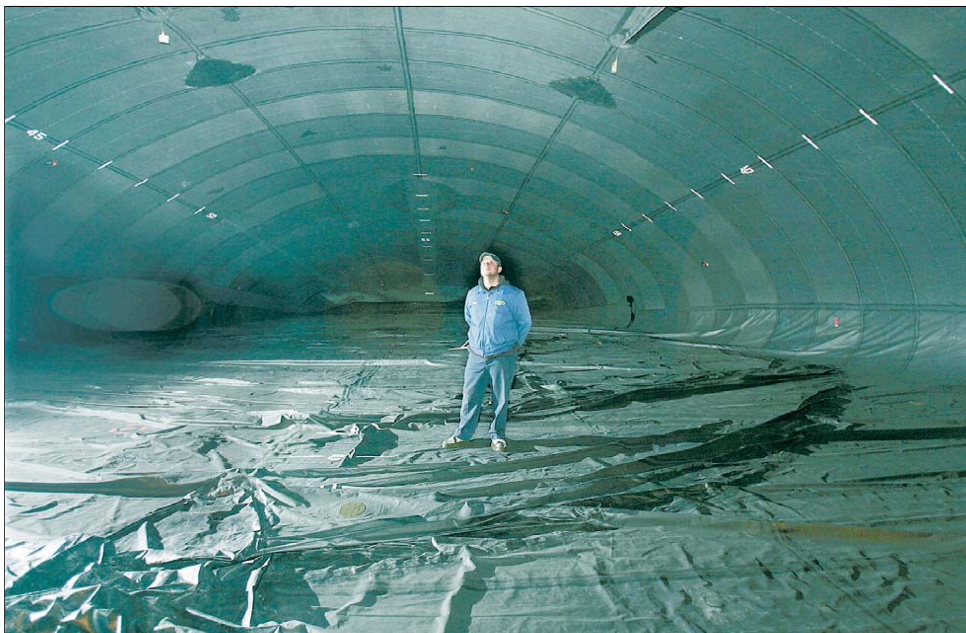
At top left, chief rigger Brian Hershberger inspects the partly inflated envelope of the unnamed Goodyear blimp being built in the Wingfoot Lake hangar in Suffield Township.
