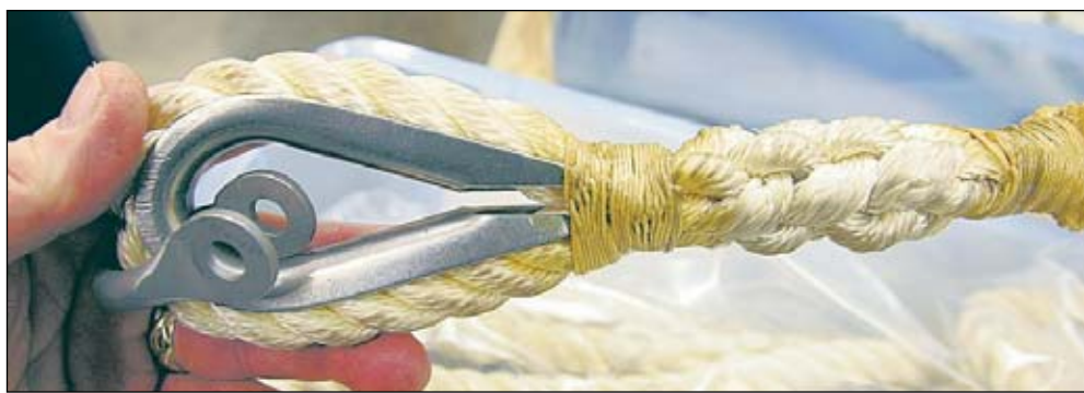
This rope is used by the ground crew to keep the blimp connected to airfield mooring masts.
