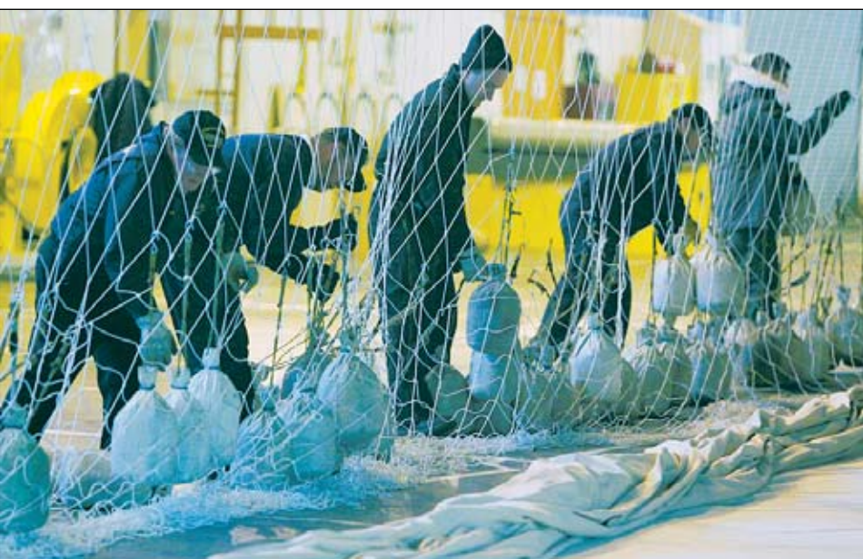
Blimp crew workers adjust the 35-pound sandbags holding a net in place during the helium inflation of the new airship at Blimp Base One in Suffield Township.
